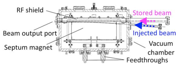
Figure 5: Schematic of in-vacuum pulse septum magnet.
