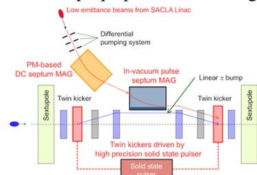
Figure 1: Schematic of in-vacuum transparent off-axis beam injection.
