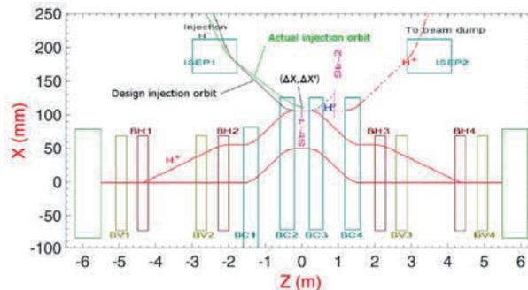
Figure 1: Physics design layout of CSNS injection system.
