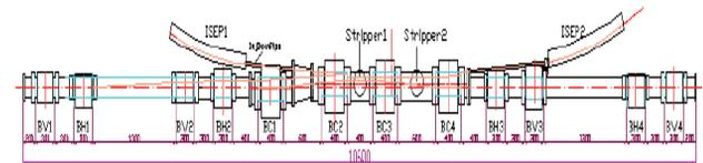
Figure 6: Machine layout of CSNS injection system.
