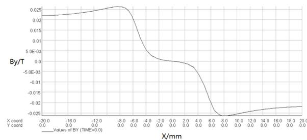
Figure 3: Simulation by OPERA2D and the magnetic field line Distribution in the NLK.
