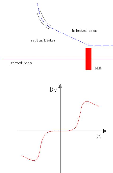
Figure 1: The layout of single pulse nonlinear kicker injection (the injected beam is deflected by the septum magnet into the NLK) and a diagram of magnetic field distribution in NLK.
