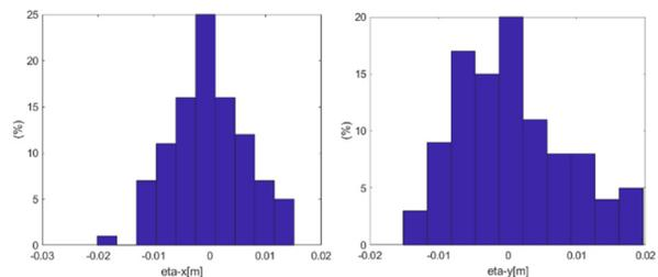
Figure 7: Distribution of dispersion at booster injection point. Left: dispersion in the horizontal plane. Right: dispersion in the vertical plane.
