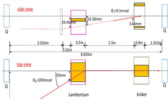
Figure 2: Layout of low energy injection system.
