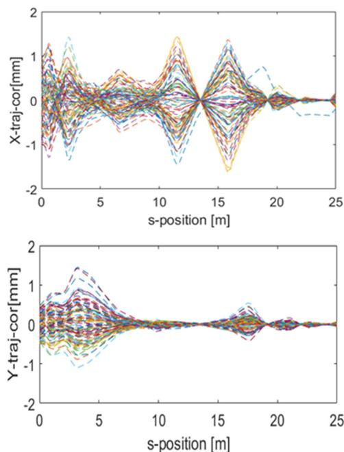
Figure 5: Beam orbit with correction. Top: Beam orbit in the horizontal plane. Bottom: Beam orbit in the vertical plane.
