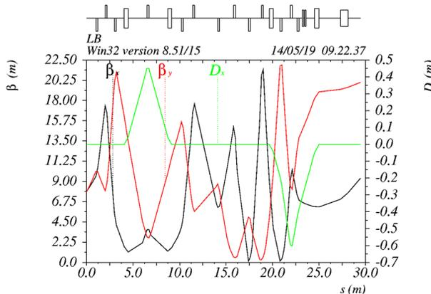
Figure 3: Lattice layout and optics parameters of LB transport line.
