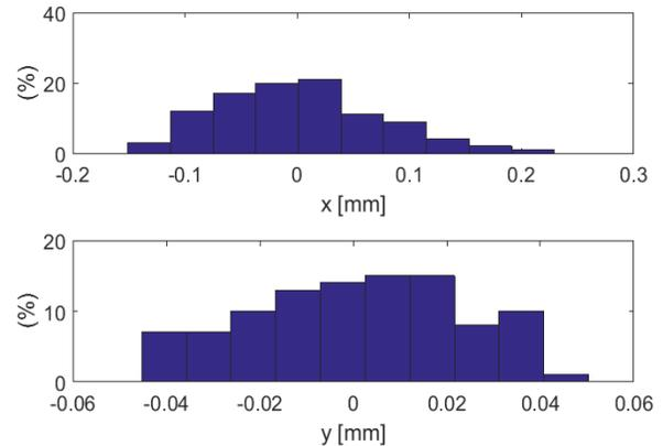
Figure 6: Distribution of beam position at booster injection point.
