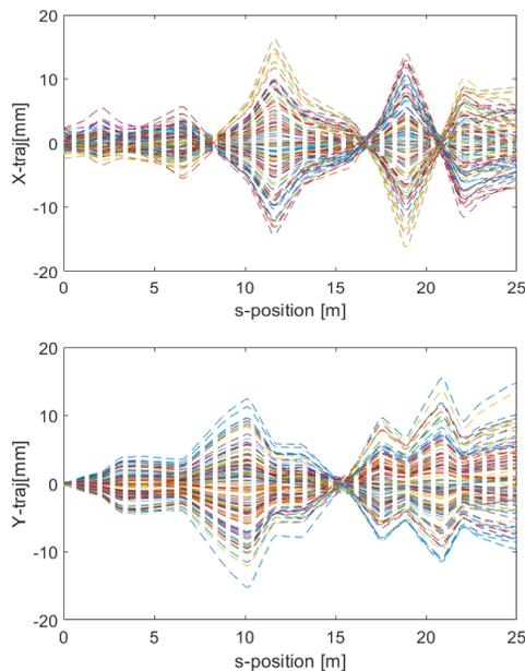
Figure 4: Beam orbit without correction. Top: Beam orbit in the horizontal plane. Bottom: Beam orbit in the vertical plane.
