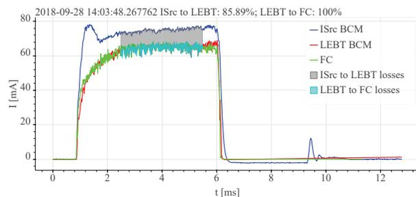
Figure 2: Beam Transmission Measurements - September 2018.
