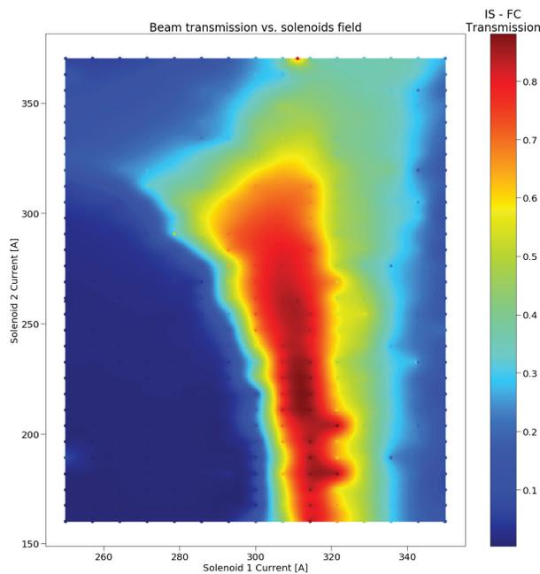
Figure 6: Transmission vs. solenoids.
