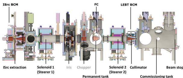
Figure 3: ESS Ion Source and LEBT Layout - March 2018.
