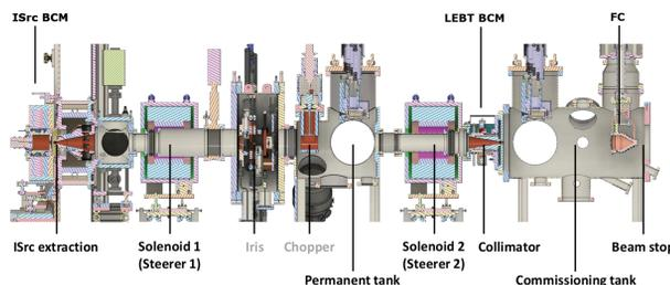
Figure 1: ESS Ion Source and LEBT Layout - September 2018.
