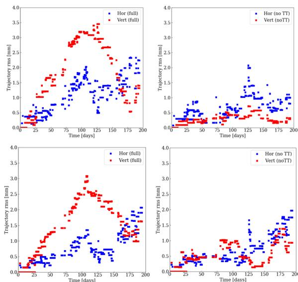
Figure 5: RMS trajectory evolution in 2018, after unfolding correction kicks. The two top plots show unfolding the corrections all over the TI 2 line (left) or only the downstream part which means leaving TT60 corrections in (right). The two bottom plots show the TI 8 trajectories, all unfolded (left) and only downstream part unfolded (right).
