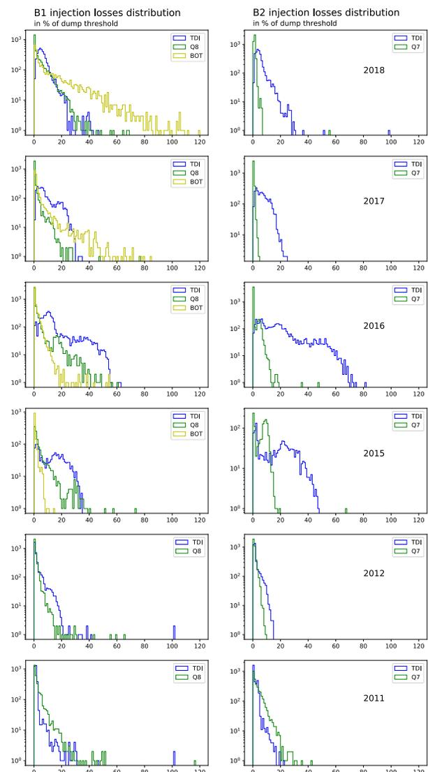
Figure 1: Distribution of injection losses for B1 (left column) and B2 (right column) from 2018 (top row) going backwards to Run 1. Transverse losses on Q8 and Q7 are shown in green, longitudinal losses on the TDI in blue.
