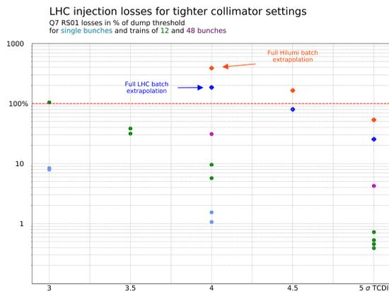
Figure 4: LHC B2 transverse injection losses on Q7 for different collimator settings and beam types.
