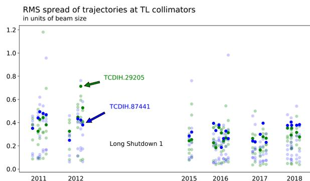
Figure 3: Spread (rms) of trajectories at TI 2 collimators (green) and TI 8 collimators (blue) in units of beam size at the respective collimator. The two critical collimators causing most of the shower on the ring loss monitors are shown in solid colours.
