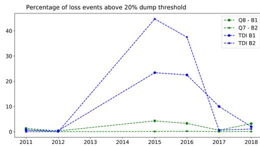
Figure 2: Percentage of injections with losses above 20% of the dump threshold, longitudinal losses in blue, transverse losses in green.
