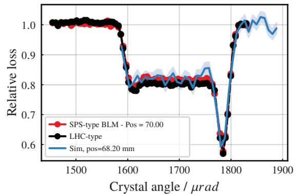
Figure 4: Relative beam loss measured on the BLMs next to the ES during an angular scan of the crystal with it positioned to shadow.
