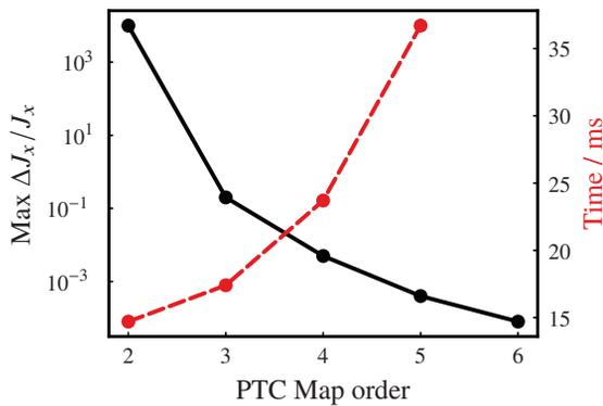
Figure 1: Comparison of tracking using sector maps extracted at different order from PTC and element-by-element tracking with MAD-X PTC at 20<sup>th</sup>-order.
