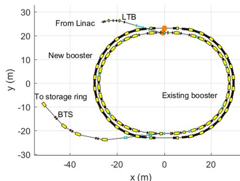
Figure 6: Location of the new booster super-imposed on the existing injector complex.
