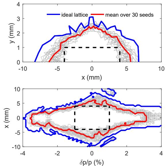
Figure 1: Impact of field and alignment errors on the on (top) and off (bottom) momentum dynamic apertures for the Diamond-II storage ring. The space available for the injected beam is highlighted in black.
