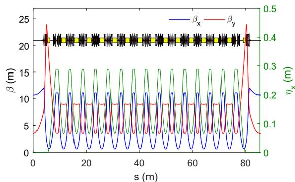
Figure 4: Twiss parameters for one super-period of the new booster design.
