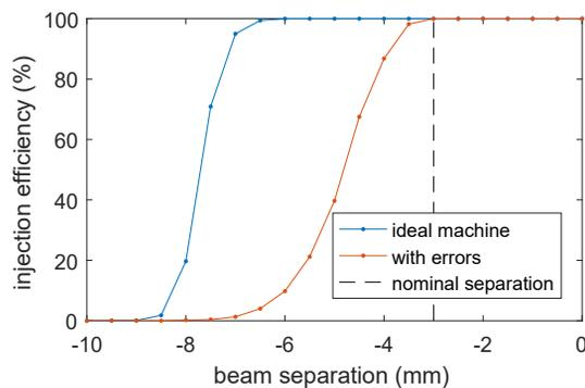
Figure 3: Injection efficiency as a function of beam separation assuming upgraded booster parameters, with and without field and alignment errors.
