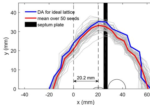
Figure 5: Dynamic aperture including field and alignment errors for the proposed booster design. The effect of the injection bump, damped beam and injected beams are shown.
