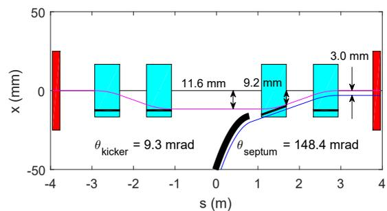
Figure 2: Diamond-II storage ring injection straight layout. Kickers are in cyan, quadrupoles are red and the septum / anti-septum plates are black curves.
