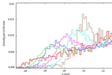
Figure 7: Evolution of the spatial density in the extracted beam during the spill. The red curve shows the distribution for the standard design configuration.
