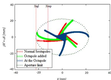
Figure 2: Phase space with an addition of an octupole magnet at the optimal location. Red shape shows the regular case (no octupole). Green and blue shapes show the phase space at the locations of the septum and the octupole.
