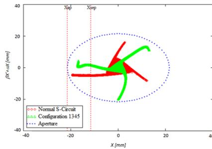
Figure 5: Extraction phase space with modified powering scheme in the standard sextupole configuration. Dash line shows the machine acceptance.
