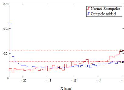
Figure 4: Extracted beam density in X. Red line shows the normal extraction, blue line shows extraction with an additional octupole. Dash lines and markers D3 and D4 are pointing to the beam density at the septum. The density D4 is reduced by 45%.
