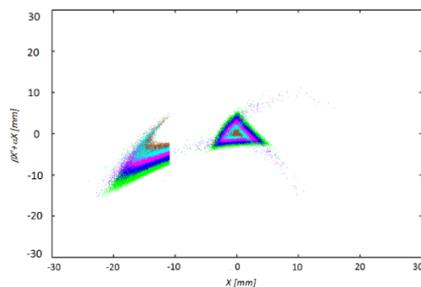
Figure 6: Separatrix shape evolution during the entire spill. Colors show the phase space at different moments of the spill.
