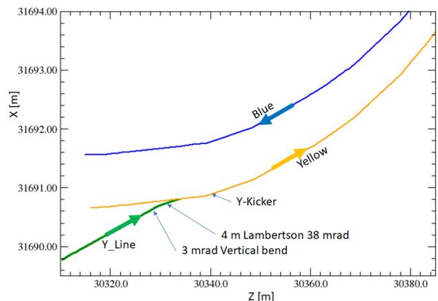
Figure 2: The green, yellow, and blue, traces are the "RHIC survey coordinates" at the entrance and exit of the elements which comprise the Y-Line (green), part of the Yellow ring (yellow) and part of the Blue ring (blue). The location of the 3 mrad vertical bend, the Labmertson septum magnet, and the 1.7 mrad vertically bending Y-kicker is shown on the figure.
