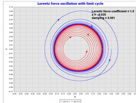
Figure 4: Limit cycle for  $x_0=0.1$  (red trajectory) and  $x_0=0.3$  (blue trajectory). The trajectory of the blue curve crosses over itself due to 3rd and higher order nonlinearity.
