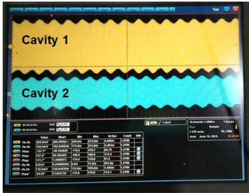
Figure 1: Experimental results showing the voltages from 2 cryomodules that have counter phase oscillations.
