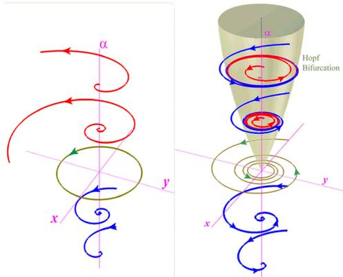
Figure 2: Trajectories for different detuning on linear and nonlinear systems due to Hopf Bifurcation.
