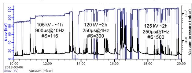
Figure 6: pulsed mode RF conditioning.
