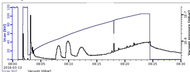
Figure 5: MP effect on the vacuum pressure.
