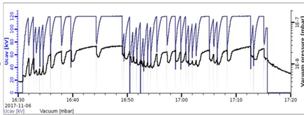
Figure 7: CW ramped RF conditioning in PLL mode.
