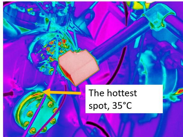
Figure 7: Infrared image of the Rebuncher at 4.3 kW power.
