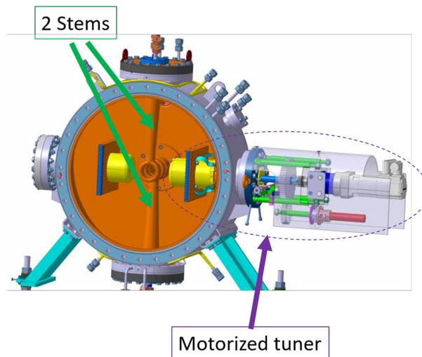
Figure 2: 3-gap rebuncher cavity components.
