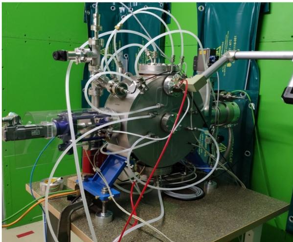
Figure 6: Fully equipped rebuncher on the RF test bench.
