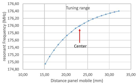
Figure 3: Frequency variation with the panel position.
