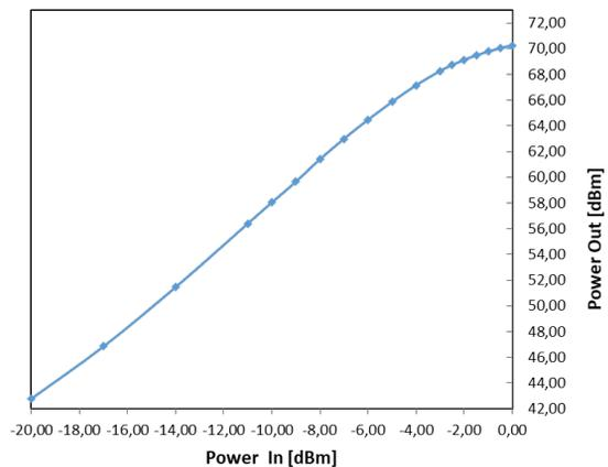
Figure 5: 10 kW RF power amplifier test result.
