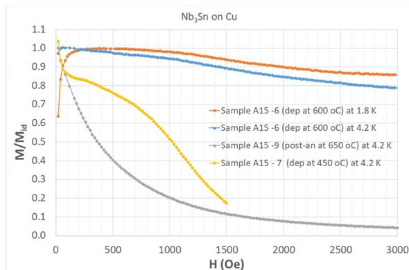
Figure 1: Normalized DC magnetization curves as a function of external applied field for Nb<sub>3</sub>Sn film deposited on copper for samples A15-6, A15-7 and A15-9.
