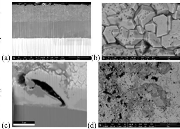
Figure 3: High resolution SEM micrograph of FIB X-section and planar view of sample A15-4 (a)-(b) pure Nb<sub>3</sub>Sn area (c)-(d) segregated copper area.
