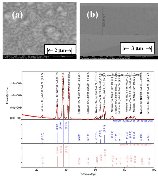
Figure 2: (a) Planar and (b) cross-section SEM micrograph, and c) the GIXRD spectrum of sample A15-6.
