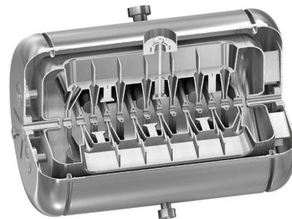
Figure 2: 3D model of the SC 217 MHz CH-0 cavity.
