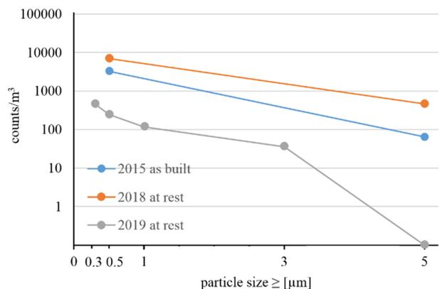
Figure 3: Particle concentrations at the “worst” spot of CR 1 during classification measurements after the CR was built (2015), altered (2018) and today.
