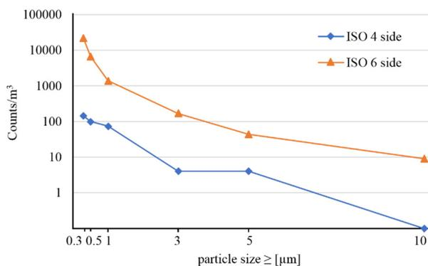
Figure 4: Measured particle concentrations during roll-up door operation inside the lock (ISO 4) and on the ISO 6 side.
