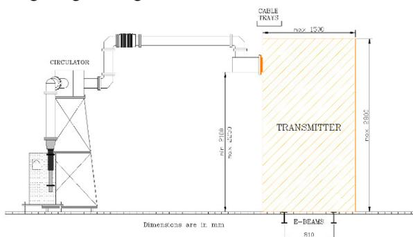
Figure 3: 100 kW with the initial coaxial line run.
