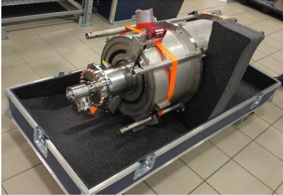
Figure 2: M001 cavity leaving Zanon. A shock logger (purple box) is visible on the top of the He Tank over the orange strap.
