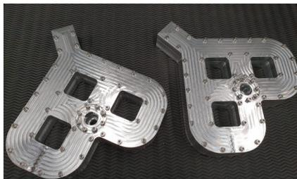
(c) Two identical fabricated MLs for back-to-back measurement.
