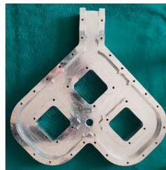
(b) Slotted plane of the Mode Launcher.
