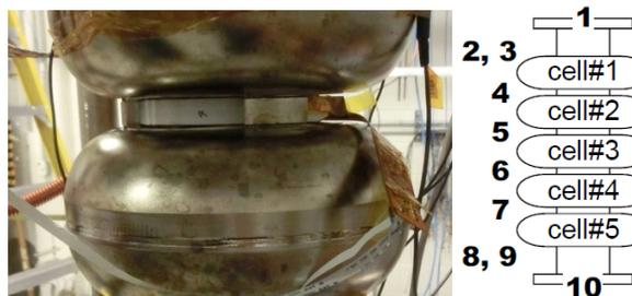
Figure 3: sX-map strip installed to cavity LSF5-1 (left). The ten strip locations are also illustrated (right).
