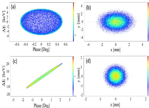
Figure 4: The particle distribution. For the input beam: (a) in phase space centered at 100 keV and (b) transversal cut in real space. For the output beam: (c) in the phase space centered on 555 keV and (d) transversal cut in real space.
