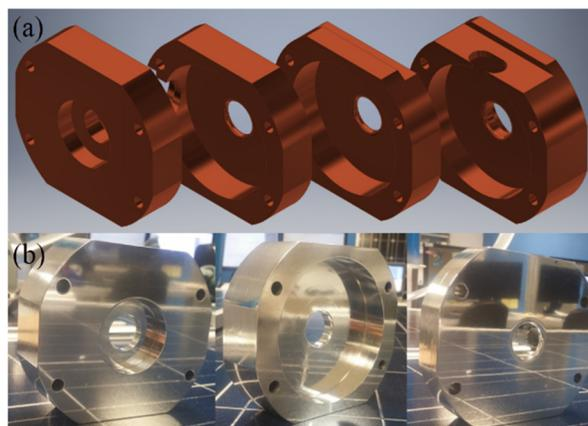
Figure 1: Mechanical design (a) and machining (b).
