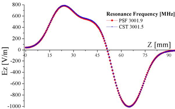
Figure 2: Longitudinal EF at  $r = 0$  for  $\pi/2$  mode.
