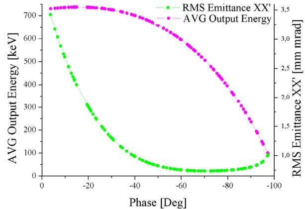
Figure 3: Variation of output energy and beam emittance when changing resonant RF electric field phase. A  $\sigma = 1$  mm beam size was used.
