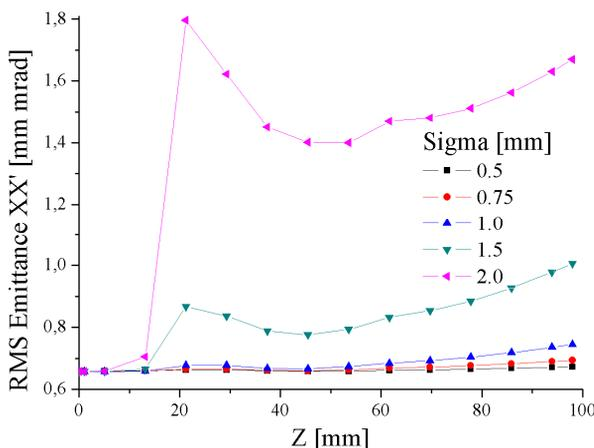
Figure 5: Emittance growth through the cavity.
