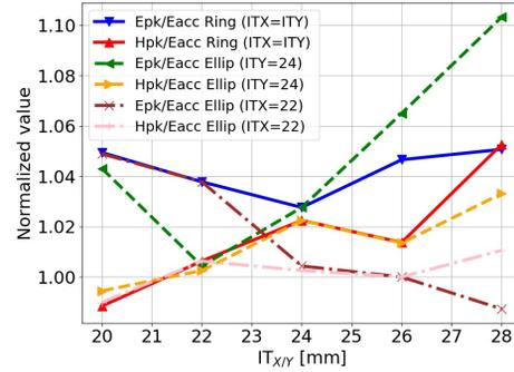
Figure 3: The values of Hpk/Eacc and Epk/Eacc as a function the transverse dimensions of the inner conductor shape. The ring shape cases (solid blue and red lines) both values were changed, and for the elliptical cases: in one ITY was fixed to 24 mm (dashed green and orange lines) and the other case ITX had a value of 22 mm (dashed-dotted brown and pink lines).
