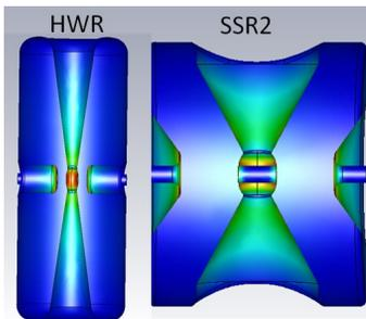
Figure 2: The electric field surface distribution for the HWR (left) and SSR2 (right). It can be seen that the higher electric fields are located in the inner center conductor (brilliant color surface).
