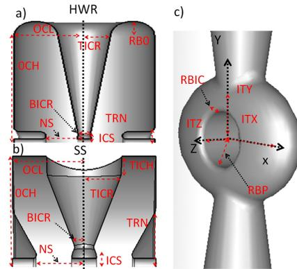
Figure 1: Parametrization of the low beta cavity geometries. On the left: a) HWR and b) SS. On the right, the inner center conductor geometry. Table 2 gives a definition of the acronyms and the final geometries values.
