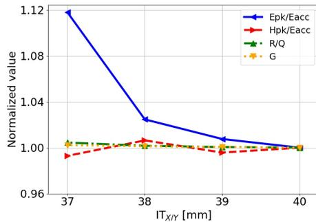
Figure 4: The figures of merits as a function the transverse dimensions of the inner conductor shape. Epk/Eacc (solid blue line), Hpk/Eacc (dashed red line), R/Q (dashed-dotted green line) and G (dotted orange line).
