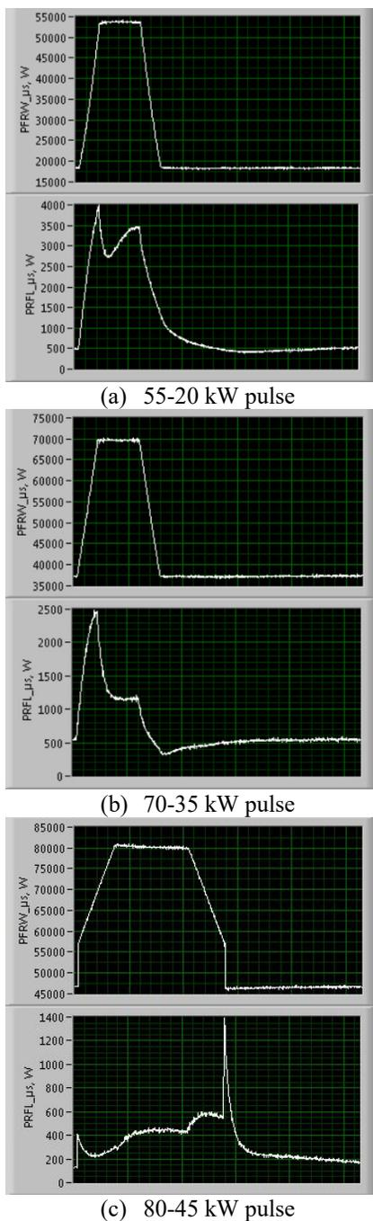
Figure 3: RF conditioning with different pulse wave.
