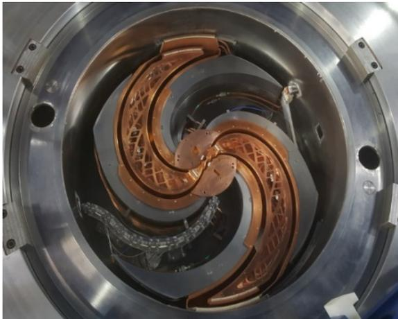
Figure 1: Assembled RF cavity in valleys.
