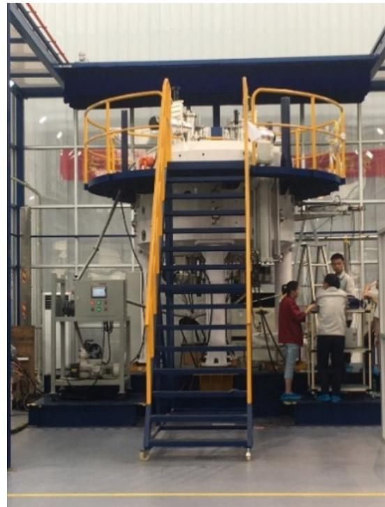
Figure 2: SC200 cyclotron host for the high-power test.
