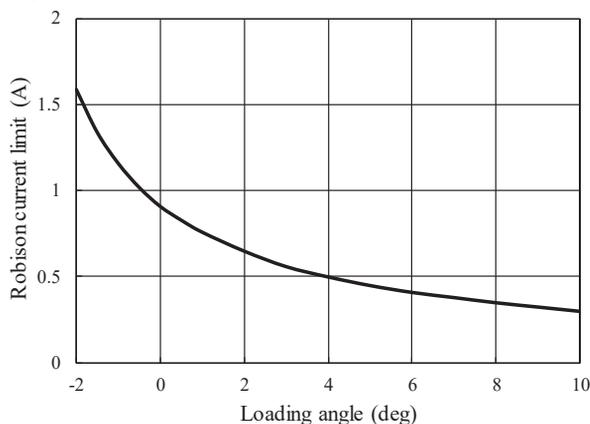
Figure 6: Robinson current limit vs. loading angle of BEPCII @ Vc of 1.5MV and beam energy of 1.89GeV.
