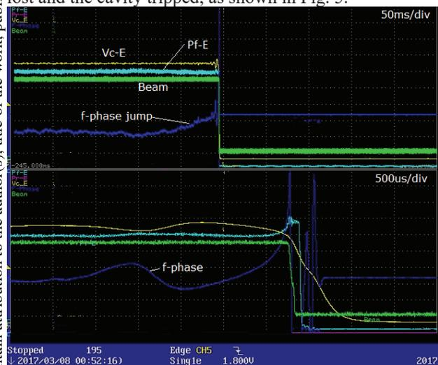
Figure 5: A typical SRF trip with the loading angle jump.
