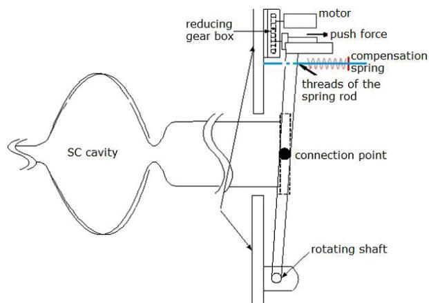
Figure 2: The schematic diagram of the BEPCII tuner.
