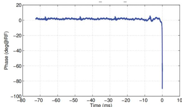
Figure 7: Beam phase monitored to be stable before the loading angle jumped and the SRF tripped.
