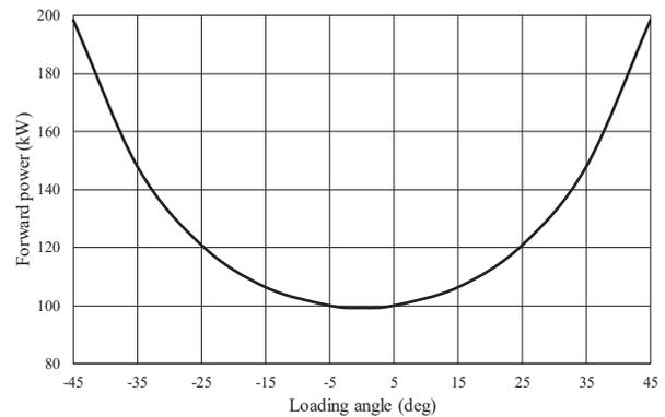
Figure 4: The forward power vs. loading angle of BEPCII @ beam current of 800mA.
