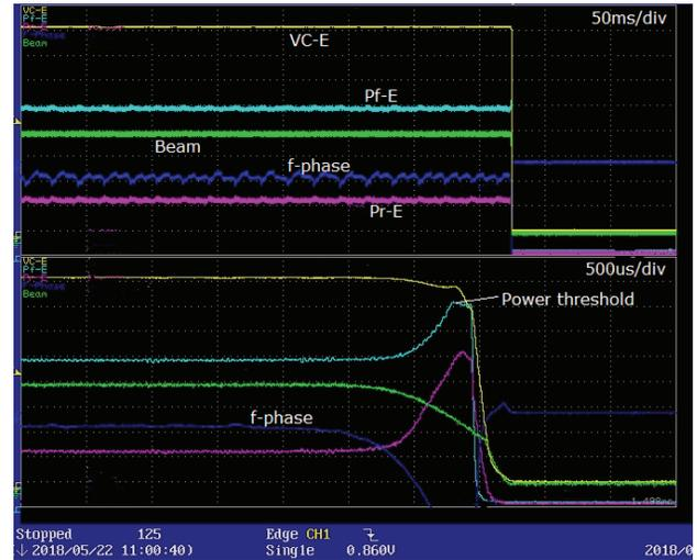
Figure 3: A typical SRF trip caused by beam loss.
