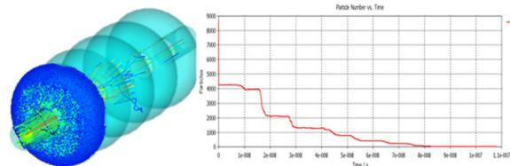
Figure 9: Particles vs. time for the end cell of the 5 cell 082 cavity.
