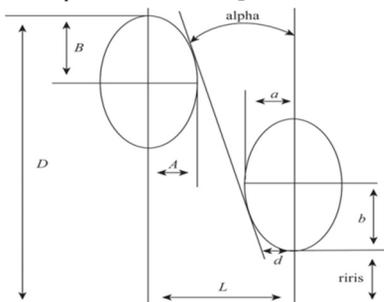
Figure 1: Schematic of the half-cell of an elliptical cavity.
