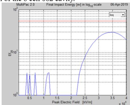
Figure 8: The final impact energy after 20<sup>th</sup> impact in the whole simulation range for the end cell of the 6 cell 062 cavity.
