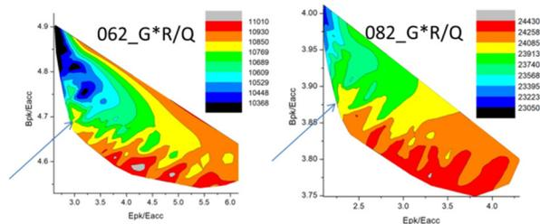
Figure 2: Contour plot of the  $G^*R/Q$  verse  $E_{pk}/E_{acc}$  and  $B_{pk}/E_{acc}$  for LB650 (left) and HB650 (right) cavities.
