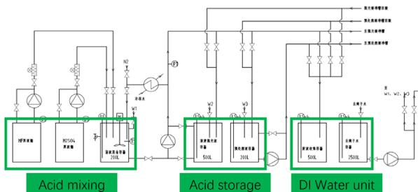
Figure 2: Schematic diagram of electrolyte preparation and equipment cleaning unit.
