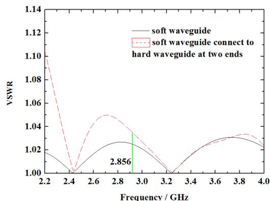
Figure 5: Frequency response of VSWR before & after adding hard waveguides.
