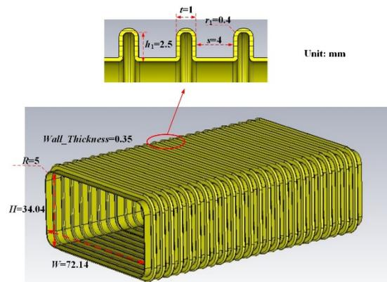
Figure 1: Detailed sizes of the flexible part of the waveguide.
