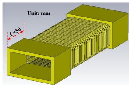
Figure 4: Simulation model with added hard waveguides.
