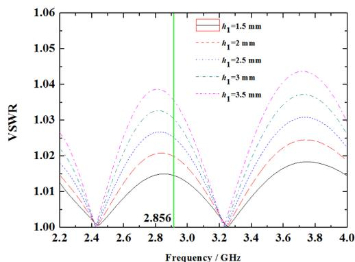
Figure 2: Frequency response of VSWR vs  $h_1$ .
