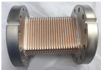
Figure 7: Picture of the flexible waveguide prototype.
