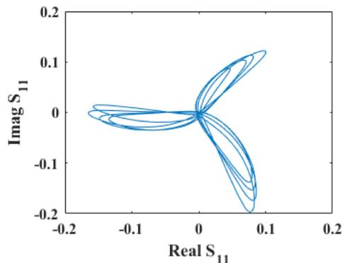
Figure 3: Complex S11 of bead-pulling.
