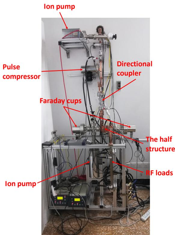
Figure 5: The half structure under test.
