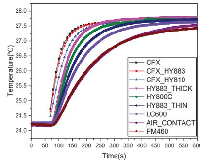
Figure 4: Temperature rising curve of different TIM in the flow outlet.
