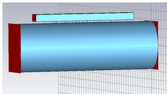
Figure 8: Circular-rectangle waveguide directional coupler in CST.
