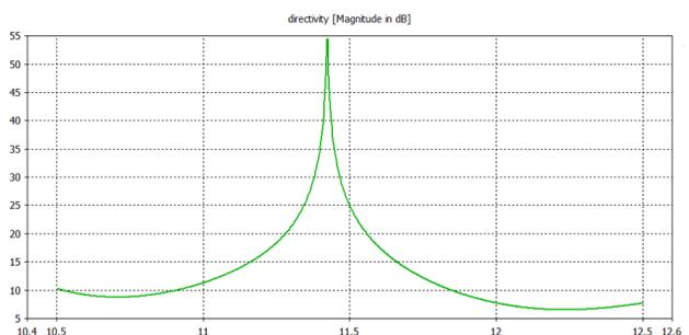
Figure 7: Directivity of H-plane directional coupler in CST.
