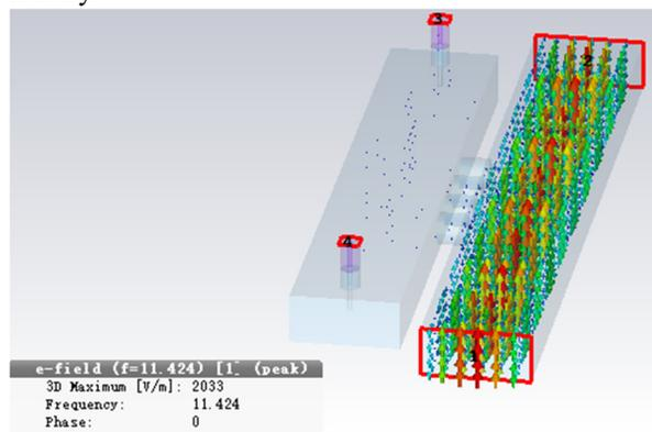
Figure 5: Electric field of H-plane directional coupler by CST.
