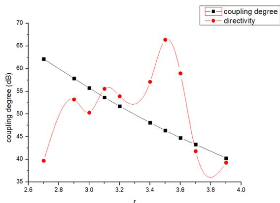
Figure 2: Curves of coupling degree and directivity with respect to the radius of the hole.
