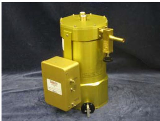
Figure 2: Bolometer detector.
