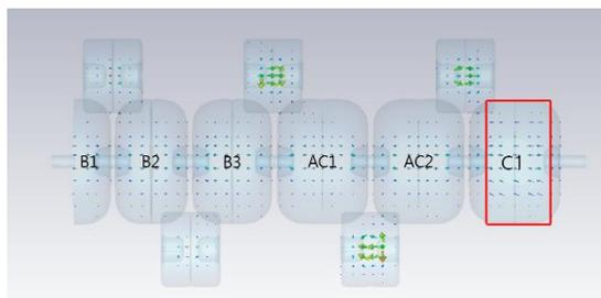
Figure 4: E-field Distribution for 1.5, 2.5 Bunching Cells.
