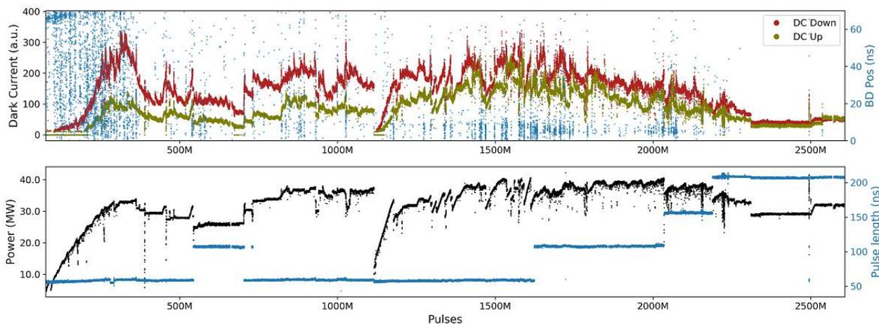
Figure 4: Full conditioning of a TD24 tested in Xbox 3. The graph in the top shows the upstream and downstream dark currents measured, together with the breakdown positioning. The one in the bottom shows the power and the pulse length.
