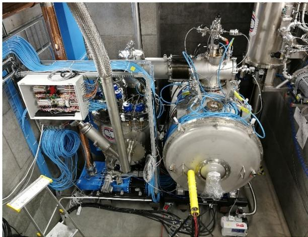
Figure 1: The ESS prototype double-spoke CM at FREIA.
