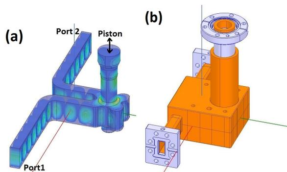
Figure 2: Phase shifter HFSS simulations (a) and general view of mechanical design (b).
