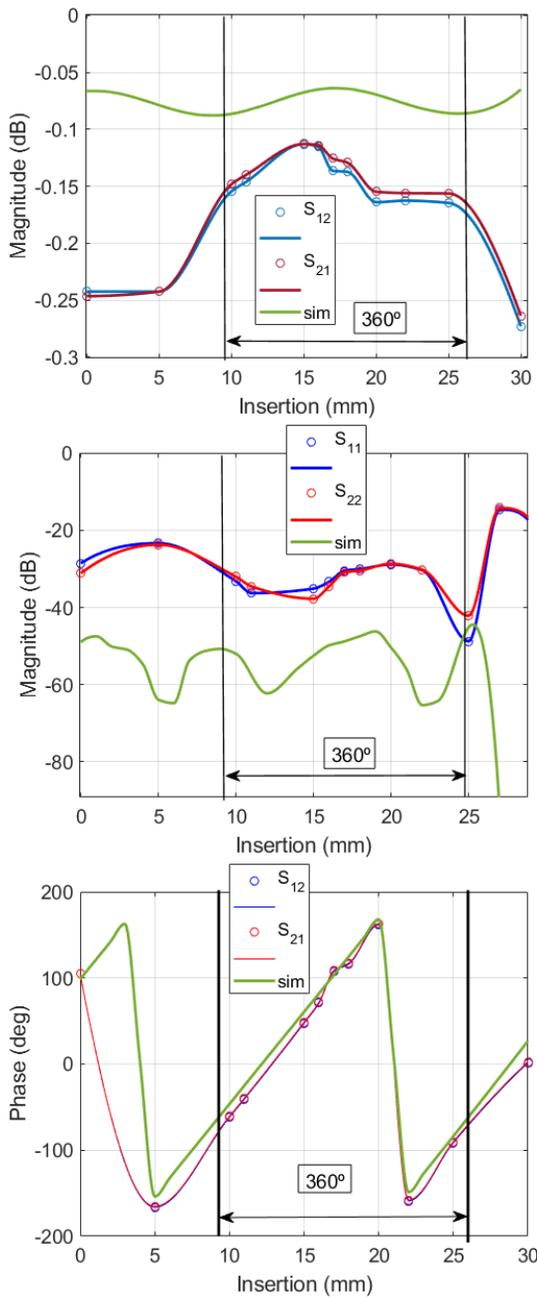
Figure 7: RF phase shifter transmission coeff. (top) reflection coeff. (middle) and transmission phase variation (bottom) vs. piston position from measurements and simulation.
