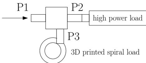
Figure 8: Schematic of the power splitter installation.
