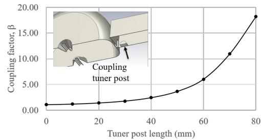
Figure 3: Power coupling tuner range of the WR-1500 waveguide coupler. Inset shows the configuration of coupling slot and the coupling tuner post.
