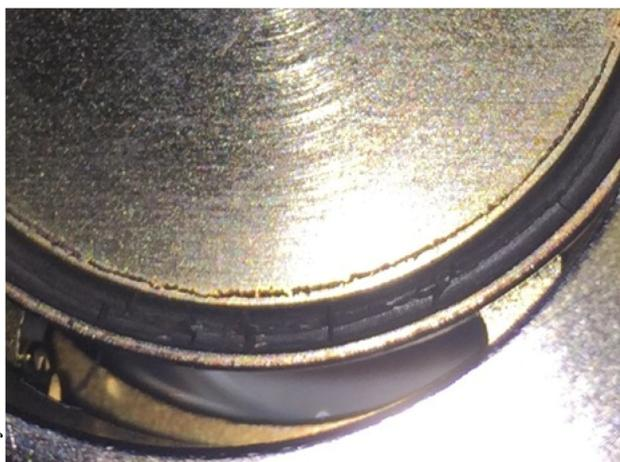
Figure 1: Cracked o-ring around the valve which occurred even with the valve open [3].
