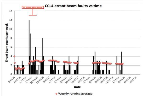
Figure 4: CCL cavity faults per week over time.
