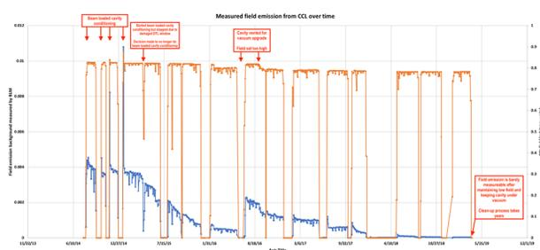
Figure 3: Field Emission measured by a BLM near a CCL cavity.
