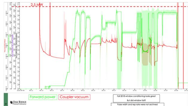
Figure 6: Conditioning Plot of Failed Window.
