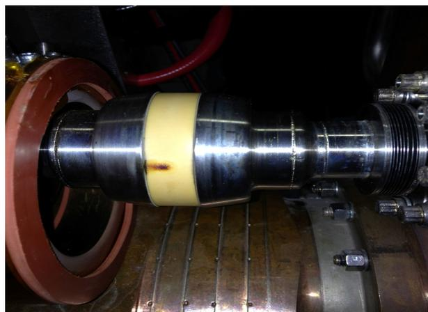
Figure 2: Electron Damage to BCM Ceramic.
