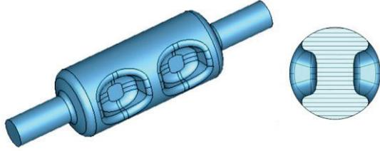
Figure 2: 952.6 MHz 2-cell rf-dipole crabbing cavity with cross section.
