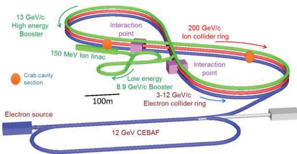
Figure 1: JLEIC electron and ion collider rings.
