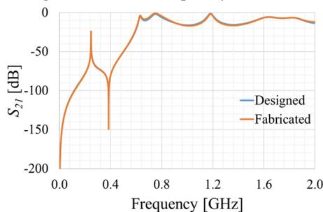
Figure 8:  $S_{21}$  transmission for the designed and fabricated rf test box.
