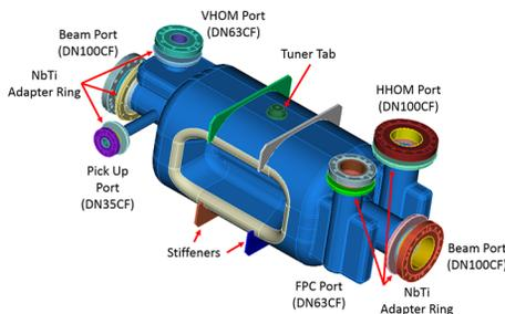
Figure 1: 400 MHz LARP prototype rf-dipole cavity.
