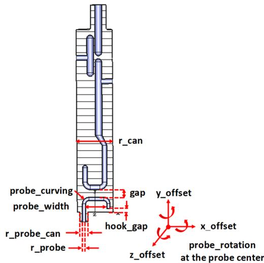
Figure 5: RF test box parameters evaluated for tolerances.
