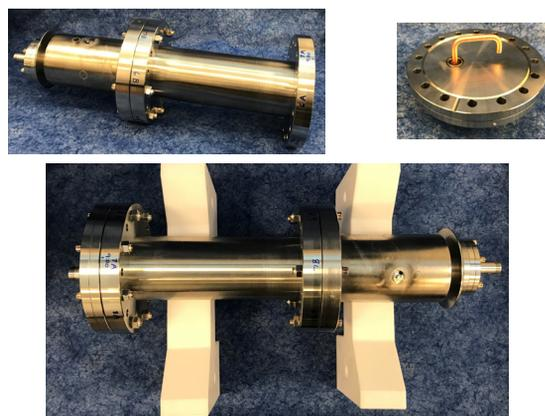
Figure 6: Test box can assembly with HHOM coupler (top left), test probe (top right), and fully assembled setup (bottom).
