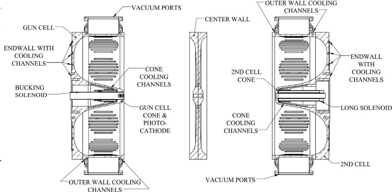
Figure 1: APEX2 cavity design.
