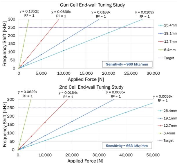
Figure 6: Endwall tuning study, frequency shift vs applied force, note that force in figure is 1/4<sup>th</sup> of required value due to symmetry boundary conditions in analysis.
