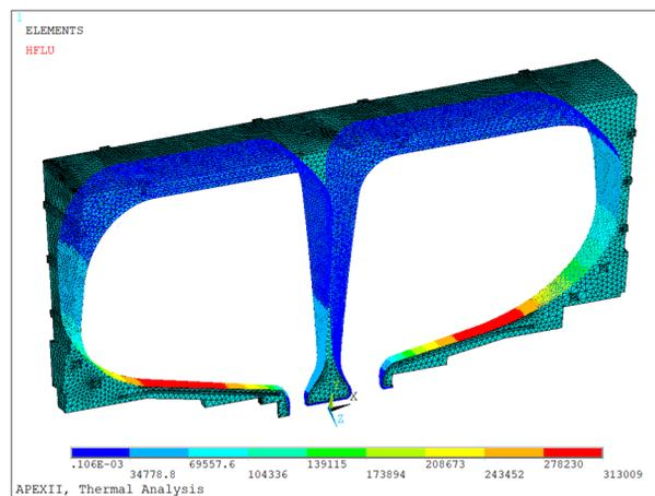
Figure 4: Cavity wall heat flux (W/m<sup>2</sup>).
