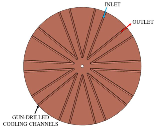
Figure 2: Gun-drilled cooling channels in the center wall.
