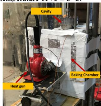
Figure 1: Set-up of 75°C baking on the waveguide insert.
