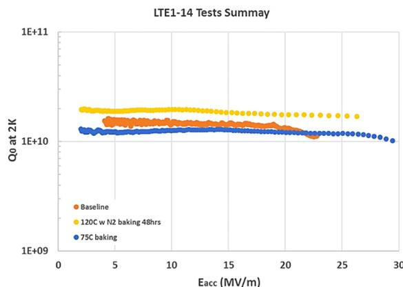
Figure 2: LTE1-14  $Q_0$  vs.  $E_{\text{acc}}$  curves at 2K.
