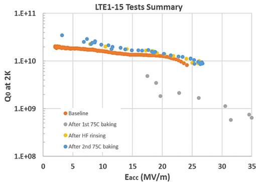
Figure 4: LTE1-15  $Q_0$  vs.  $E_{acc}$  curves.
