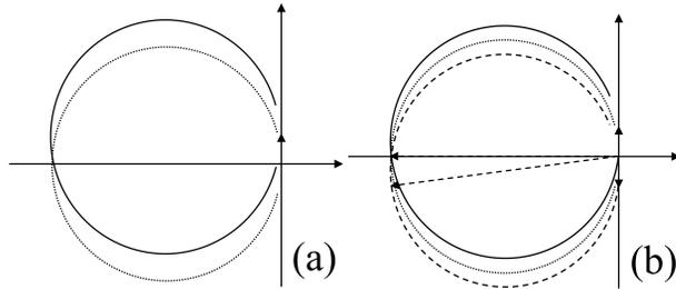
Figure 3: Polar chart of the  $S_{21}$  (a) at room temperature (b) at cryogenic temperature. With dotted circle the cavity resonance without crosstalk, and the solid circle with. The dashed circle in (b) represents the rotation and enlarging of the circle.
