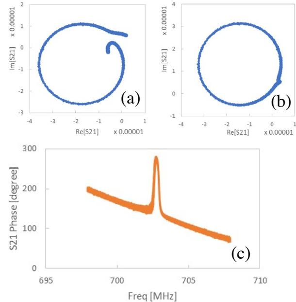
Figure 4: (a) Measured Re-Im chart of the  $S_{21}$ ; (b) Re-Im chart after considering phase on coaxial/waveguide cables; (c) Measured  $S_{21}$  that shows the phase versus frequency.
