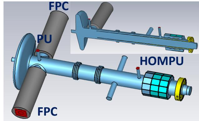
Figure 1: LEReC booster cavity with cross-section view (top-left).
