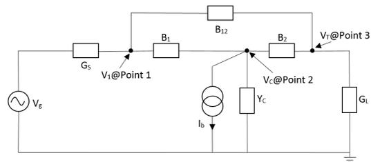
Figure 2: Circuit model of the cavity with crosstalk.
