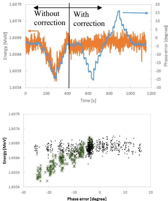
Figure 5: (top) Measured beam energy without (<400s) and with (>400s) crosstalk correction, while intentionally detuning the cavity resonance frequency. (bottom) Energy versus phase error without (green star) and with (black dot) crosstalk correction.
