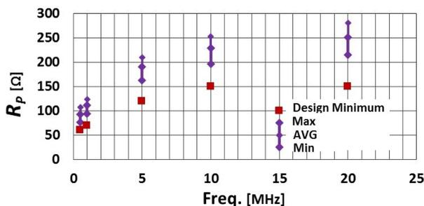
Figure 4: MA Cores Loss Resistance  $R_p$ .
