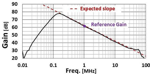
Figure 7: Power Amplifier Frequency Response.
