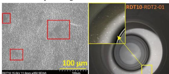
Figure 5: RDT10-RDT2 coating. SEM image [left] shows patchy regions observed in witness sample. Non uniformity in the coating can be seen in the right picture. Note that the top half cell had less non uniformity than the bottom.
