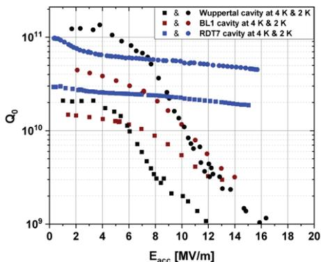
Figure 4: Comparison of RF results from RDT7 with previous data with Q-slopes.
