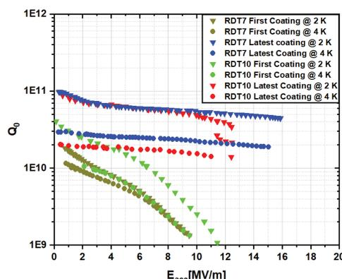
Figure 7: Comparison of latest RF test results from RDT10 and RDT7 with those after their first coating. RDT10 is expected to have higher Q<sub>0</sub> at 4 K than presented here as we expect losses on the flanges because of shorter beam pipes.
