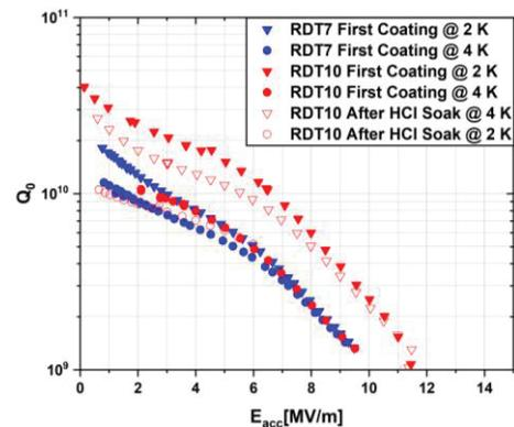
Figure 3: RF test results from RDT7 and RDT10 after first  $\text{Nb}_3\text{Sn}$  coating. Note that RF results following 5 % HCl soak are also shown.
