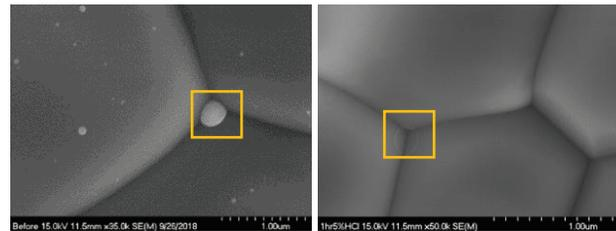
Figure 2: SEM images from RDT7 witness sample before [left] and after [right] 5 % HCl soak for one hour. Bright features are Sn-rich residues.
