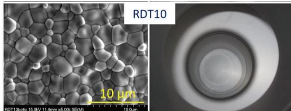
Figure 1: SEM image captured from RDT10 witness sample is shown on the left. Right image is the appearance RDT10 after coating [right].
