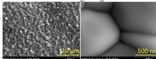
Figure 6: SEM images from RDT10-RDT2 coating. Note that there is Sn residue in the surface [right].
