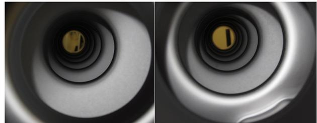
Figure 1: A picture of the inside of IA110 coated with Nb<sub>3</sub>Sn. The left picture is taken through the beam tube on the fundamental power coupler side, which is at the bottom during coating. The right picture is taken through the beam tube on the high order mode couplers side, which is at the top during coating. Note similar coating appearance at both sides.
