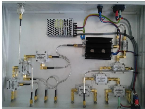
Figure 2: Inside of the MO divider.
