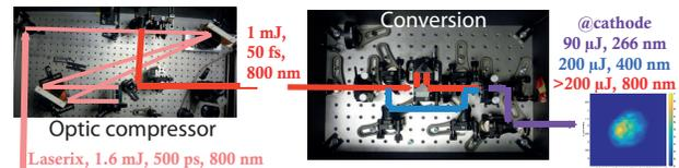
Figure 1: Schematic of the pulse compressor and the frequency conversion of the Ti:Sa laser LASERIX for the 3GHz RF gun cathode
