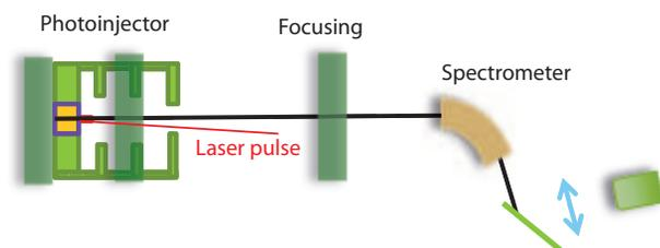
Figure 2: schematic of the PHIL test line used for the DRUM experiment. The laser pulse is send to the cathode in the RF gun. Different solenoids are allowed for focusing a spectrometer combined to a YAG screen and imaging are available for energy spread measurements
