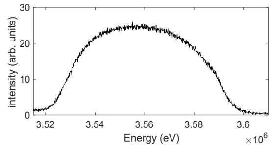
Figure 3: top : image of the YAG screen after the spectrometer. bottom, energy distribution profile of the electron bunch. Both cases are in the case of short laser duration at the cathode illuminated by UV light.
