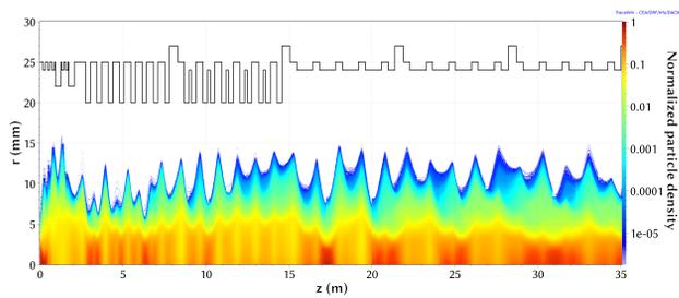
Figure 2: Beam density in  $r$  plane along the DONES SRF-linac.
