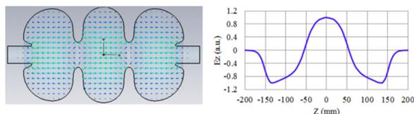
Figure 4: Electric field array plot and variation in on-axis accelerating of  $\pi$  mode in three-cell buncher predicted by CST MWS.
