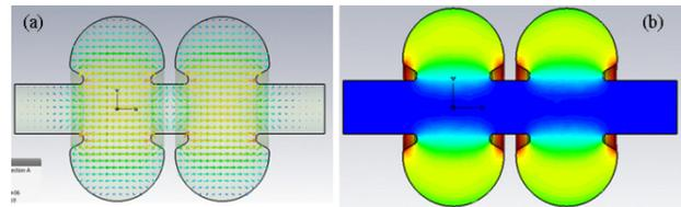
Figure 1: Two-cell buncher (a) electric field array plot and (b) magnetic field distribution for  $\pi$  mode predicted by CST MWS.
