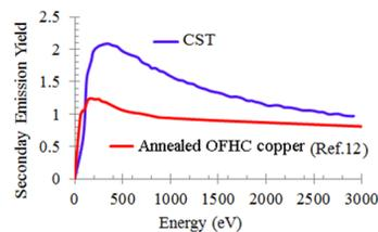
Figure 6: Comparison of SEY of copper given in CST and in reference [12].
