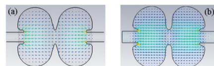
Figure 2: Shape of (a) tapered (DESY design 1) and (b) elliptical (DESY design 2) inter-cell coupling iris.
