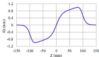
Figure 3: Variation in on-axis accelerating field for the two-cell buncher with elliptical inter-cell coupling iris.
