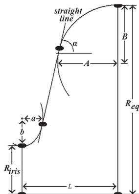
Figure 8: Schematic diagram of half of central cell, picture taken from [9].
