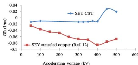
Figure 9: Exponential growth rate as a function of voltage in the three-cell buncher predicted by CST PS tracking solver.
