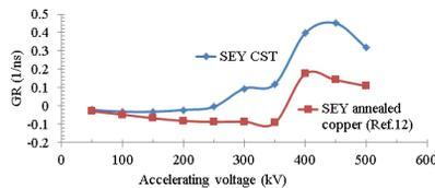
Figure 7: Exponential growth rate as a function of voltage in the three-cell buncher predicted by CST PS tracking solver.
