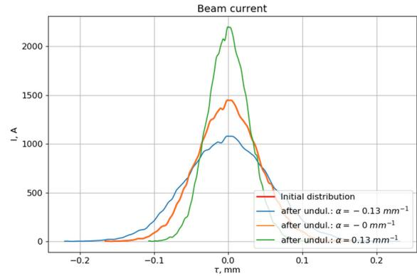
Figure 2: Beam current after THz undulator.
