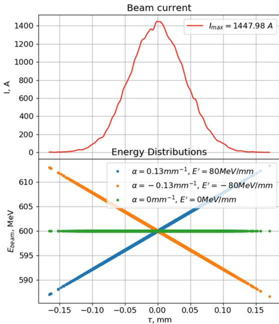
Figure 1: Energy distribution and beam current in front of THz undulator.
